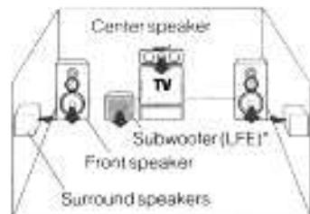
\*LFE = Low Frequency Effects. This channel delivers separate non-directional bass signals to the subwoofer for more dynamic deep bass sound effects.
