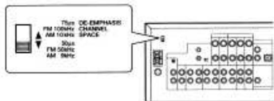
Move switch lever to match your area with a small screwdriver or other pointed tool.
