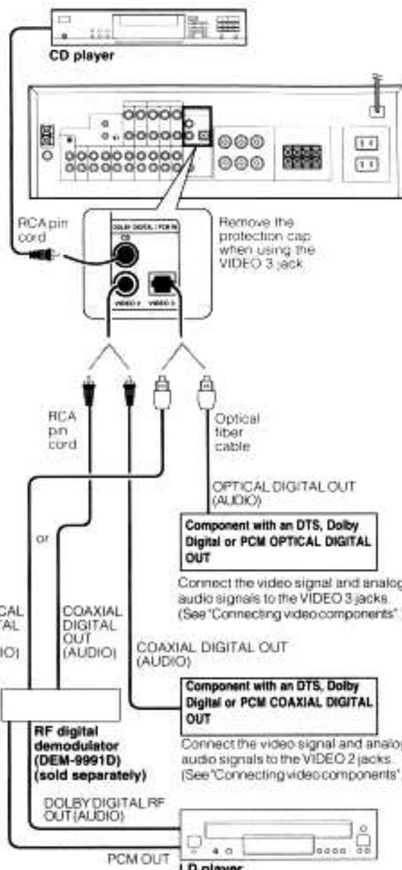
To connect an LD player with a DIGITAL RF OUT, connect the LD player to the KENWOOD RF digital demodulator (DEM-9991D). Next, connect the DIGITAL OUT jacks of the demodulator to the DIGITAL IN jacks of the receiver.
